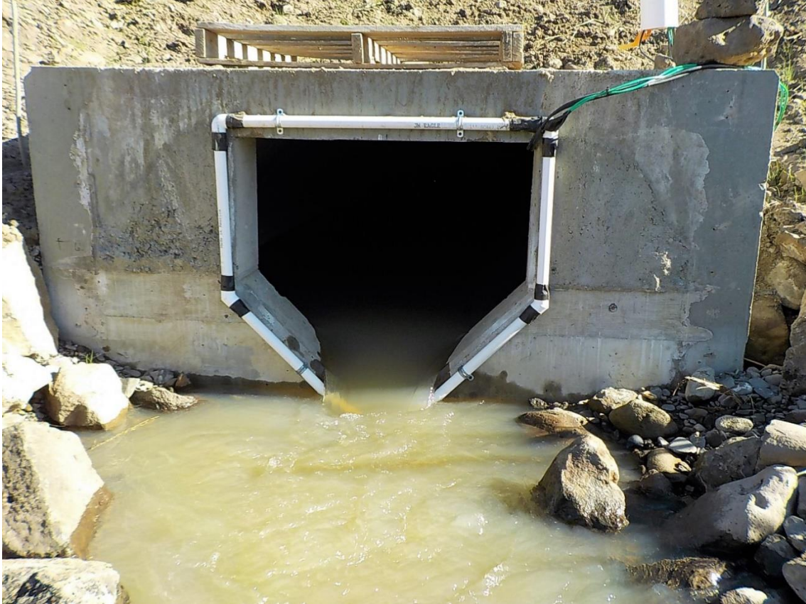
Figure 2. The V-notch weir and loop PIT antenna on the downstream end of box culvert at the MC Diversion fish passage project. Photo taken on 03 May 2018.
