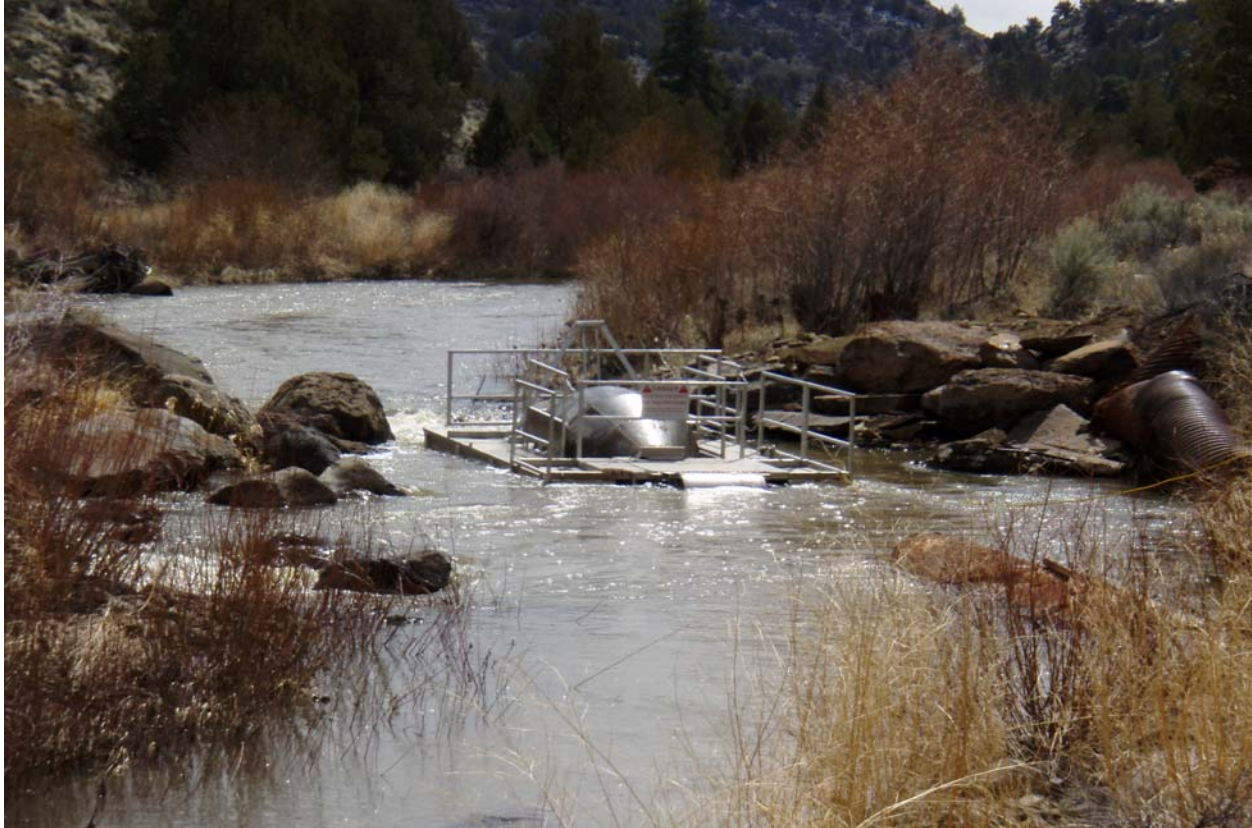
Figure 5. Downstream migrant screw trap fished in Twelvemile Creek, 2008. The trap was located 2.5 km upstream of the confluence with Twentymile Creek at the site of the former O'Keefe diversion.
